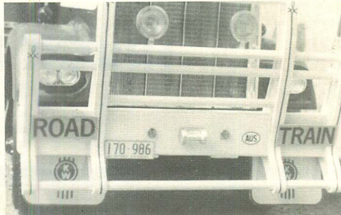
Front of Kenworth with scratch built bull bar, photo reduced number plate and mudflaps, driving lights from AMT. A model Roadster.
