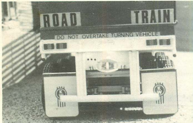
Photo reduced mud flaps, ringfeder rams horns for dolly safety chains.
